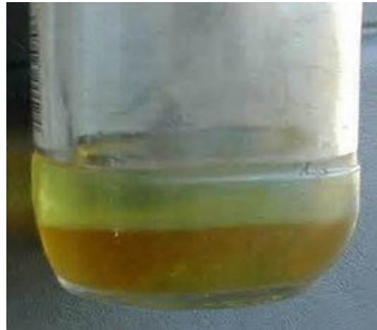
Diesel fuel sample showing water and sediment contamination.
