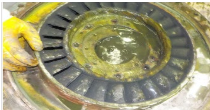
Figure 2: Turbocharger Nozzle Ring fouling
